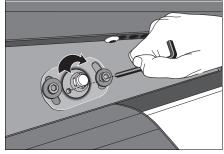
Figure 8: Wheel lock adjustment
