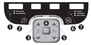
**Diagram 4: Lower Display keypad and the Selection keys**
