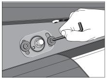
Figure 7: Loosen the two adjustment screws
