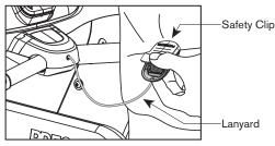
Figure 3: Attaching the safety clip
